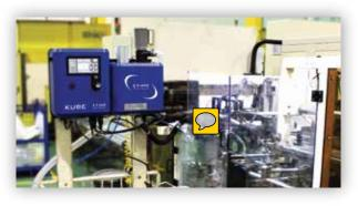
Engineered to operate with three different mount configurations, the Kube is suitable for both new machine installations, as well as system upgrades/ replacements.
